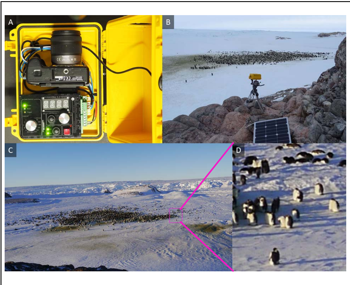
Fig. 1: micRObs recording system in the field. (A) The camera housing contains the control box and camera. (B) System deployed in the field at Pointe Géologie archipelago, Adélie Land, Antarctica ( 66^{\circ}42'01''S 139^{\circ}49'41''E , May 2019). The camera housing is mounted on a tripod with a pan/tilt ball mount. The system is powered by a 12 V car battery with a solar panel and charge regulator. (C) Image recorded with micRObs. (D) Enlarged detail: Individual animals are clearly distinguishable.
