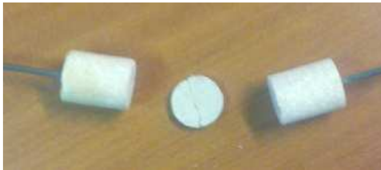
Figure 18: Specimen A failure in tension.
