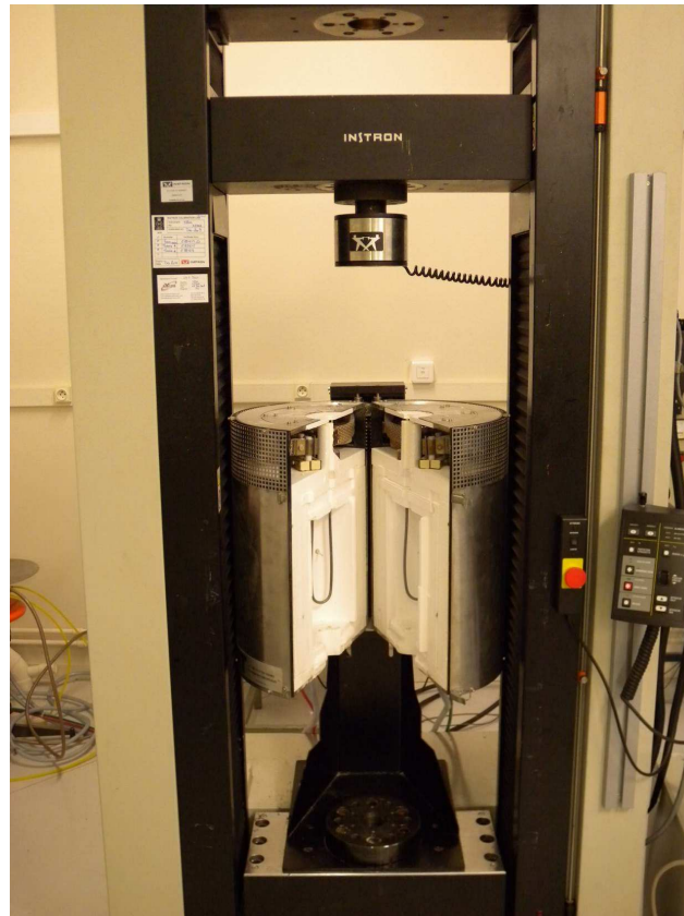
Figure 13: Universal testing machine with the furnace (AET ref. OF 25 957 Type SP)
