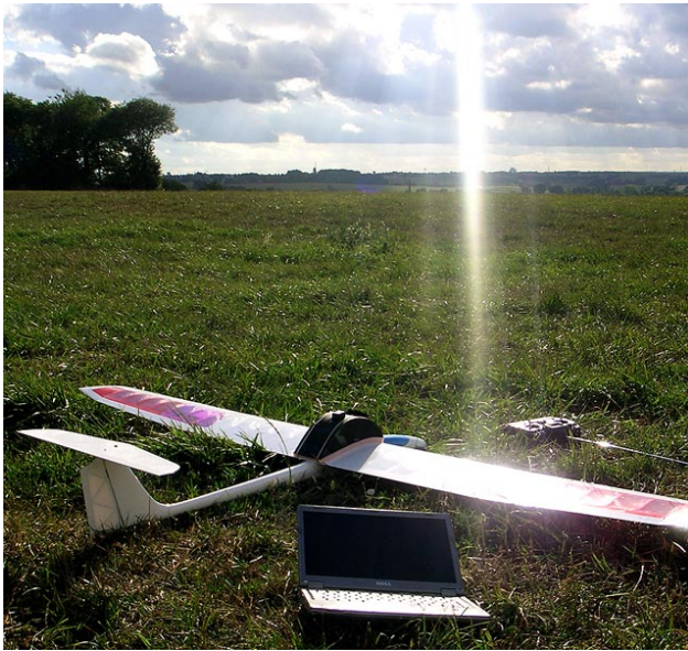
Figure 8. Motor-glider under development to test thermal and slope soaring in real conditions.
