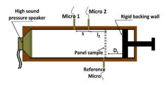
Fig. 3 – Schematic of the impedance tube used for the measurements.
