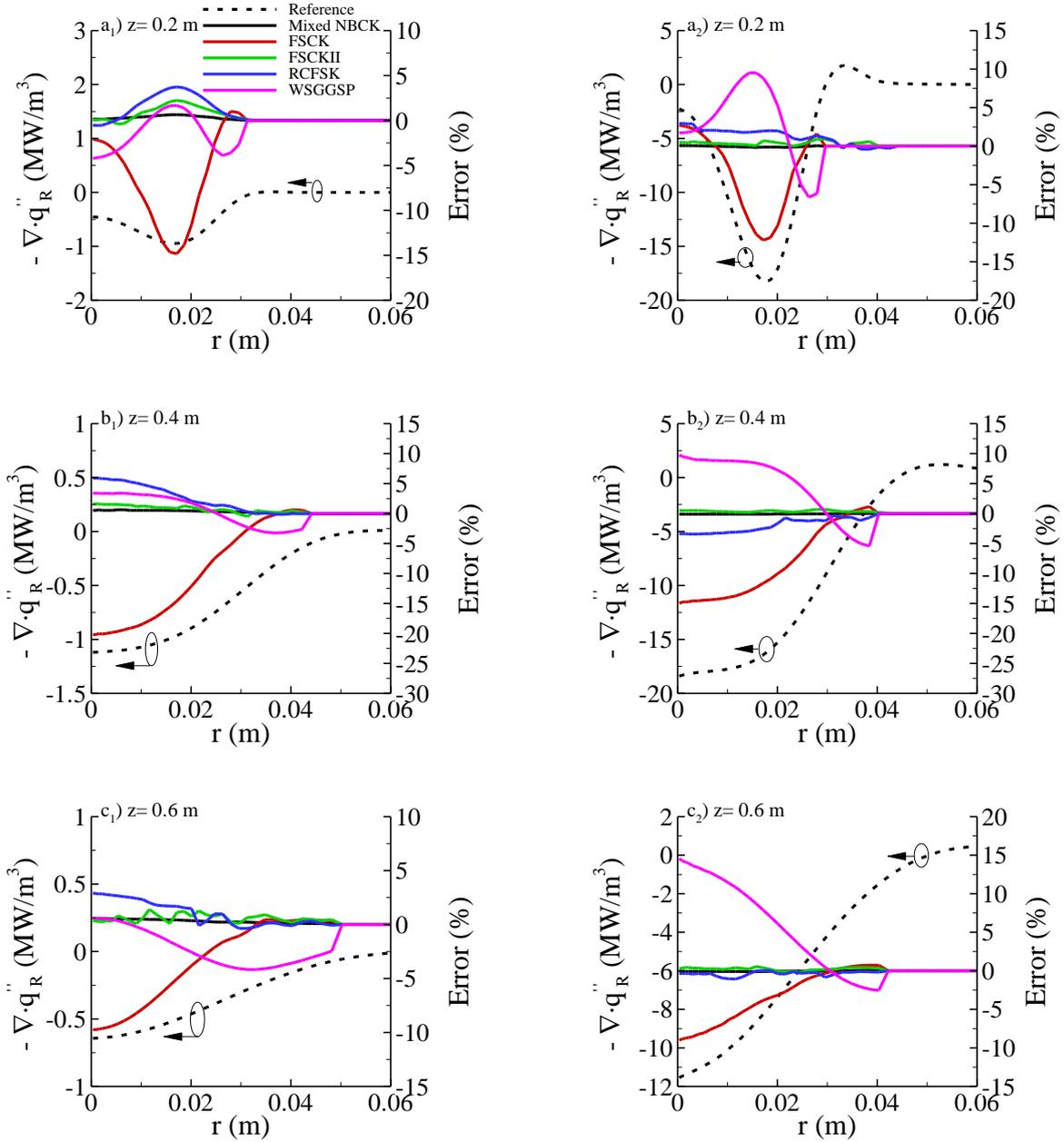
Figure 3. Radiative source term and relative error in percent as a function of the radial distance at different heights of: a) 0.2 m, b) 0.4 m and c) 0.6 m. The indexes 1 and 2 refer to the H<sub>2</sub>/air flame at 1 atm and 30 atm, respectively.
