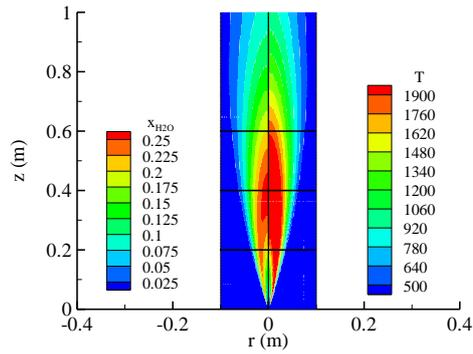
Figure 1. Fields of H<sub>2</sub>O mole fraction (left) and temperature (right) for the H<sub>2</sub>-air flame at 1 atm.
