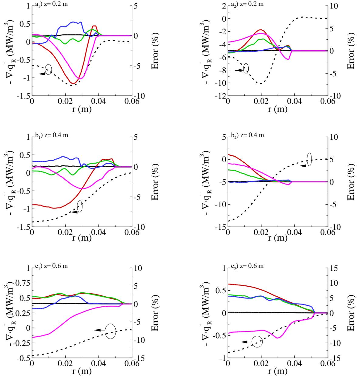
Figure 4. Radiative source term and relative error in percent as a function of the radial distance at different heights of: a) 0.2 m, b) 0.4 m and c) 0.6 m. The indexes 1 and 2 refer to the CH<sub>4</sub>/air flame at 1 atm and 4 atm, respectively. See the legend of Fig. 3.
