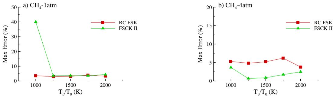
Figure 5. Effects of Planck ( $T_P$ ) / reference ( $T_0$ ) temperature on the maximum error on the divergence of the radiative flux. The abscissa axis uses  $T_P$  for the RC-SLW and  $T_0$  for FSCK II. The errors for the radiative source term are based on the three radial profiles at  $z = 0.2, 0.4$  and  $0.6$  m.
