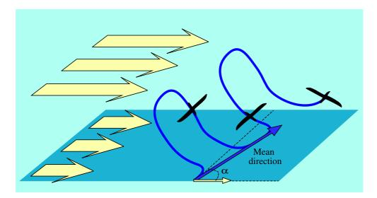
Figure 1. Trajectory used by the albatross for dynamic soaring. At the highest point of the trajectory, the albatros turns back to the wind and starts diving to gain speed. At the lowest point, the albatros sharply turns to face the wind and exploits the speed gained during the dive to gain altitude. At the end of this phase, the bird has reached the same altitude as that of its starting point. On average, the birds flies at a certain angle  $\alpha$  with respect to the wind.
