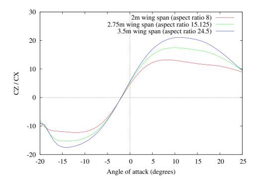
Figure 3. Variation of the lift/drag factor (CZ/CX) according to the angle of attack for the whole glider. Aspect ratios are taken into account in the calculation of the characteristic curves of each panel. The total wing area is held constant at  $0.5 \text{ m}^2$ , no sideslip effect is present here.
