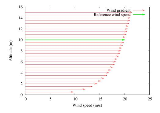
Figure 4. Wind-speed gradient used in the model
