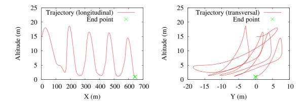
**Figure 8.** Longitudinal and transversal projections of the glider's trajectory with the reference controller (wind-speed : 20 m/s). The flight is not regular and ends after four cycles at the "End point".
