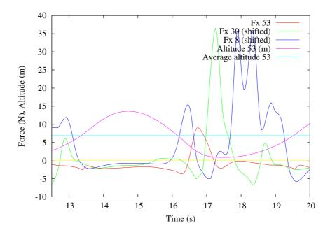
Figure 14. Resultants of aerodynamic forces projected on the longitudinal axis of the glider  $(F_x)$ .  $F_x$  is lesser with the 53° controller than with the two others. In particular, it is negative and, most of the time, smaller than the others when z is greater than  $z_{avg}$ .
