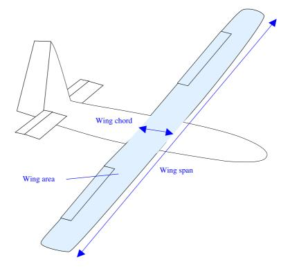
Figure 10. Characterization of the wing span, the wing chord, and the wing area that serve to calculate the wing's aspect ratio.
