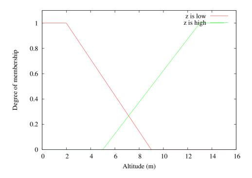
**Figure 5.** Fuzzy sets defined on variable z (altitude). Two sets are defined, respectively for high and low altitudes, the corresponding degree of membership progressively changing according to the glider's altitude. In other words, when the latter is lesser than five meters, the system's altitude has more chances to be classified as "low" than as "high".
