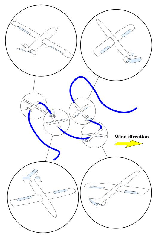
Figure 6. Glider's trajectory and position of its control surfaces in each phase. See text for details.
