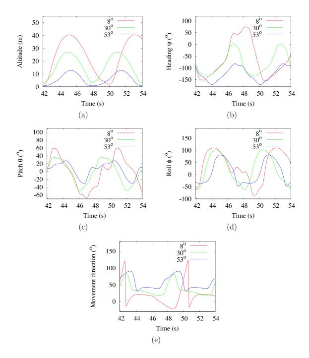
Figure 13. Altitude (a), orientation angles (heading (b), pitch (c) and roll (d)) and movement direction (e) of a glider flying toward three different mean directions :  $8^{\circ}$ ,  $30^{\circ}$  and  $53^{\circ}$  relative to the wind. Data for  $8^{\circ}$  and  $30^{\circ}$  have been respectively shifted by 2.4 s and 1.5 s, to synchronize the beginning of each cycle.
