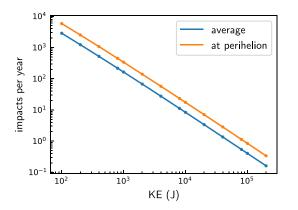
**Figure 1.** The impact rate of meteoroids on Bennu as a function of limiting kinetic energy. We find that collisions with kinetic energies of 4,000 J (4 kJ) take place approximately once every 2 weeks if we average over the entire orbit, the same cadence as the three largest particle ejection events observed to date on Bennu. If we concentrate on impacts at perihelion, where the impact rate is higher, 7,000 J (7 kJ) impacts are delivered biweekly.
