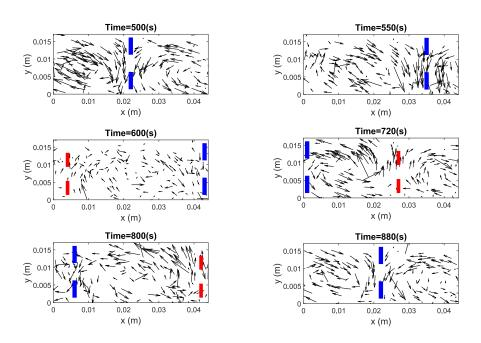
Figure 10: Velocity vectors during a period for 1/Y=16.5 - Dashed lines: approximate boundaries between two counter-rotative cells, Blue for the lower flow and Red for the upper flow. Oscillations take the form of traveling waves (TW) moving from left to right in this case  $(v_p>0)$
