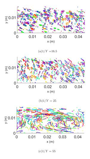
Figure 6: Trajectories obtained with TRACK in the gel ( $\tau_y=0.03$  Pa) for (a) 1/Y=16.5, (b) 1/Y=25 and (c)1/Y=55. One color corresponds to one tracked particle. For a sake of clarity, all tracked particles trajectories are not represented.
