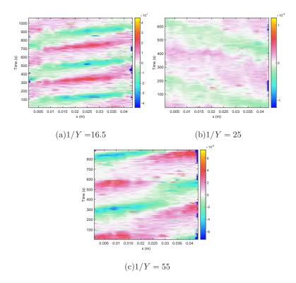
Figure 11: Space-time diagrams (a)-(c) showing the evolution of the midplane vertical velocity  $v_y$  as a function of location x obtained in the gel ( $\tau_y = 0.03 \text{ Pa}$ ) for (a) 1/Y = 16.5, (b) 1/Y = 25 and (c) 1/Y = 55.
