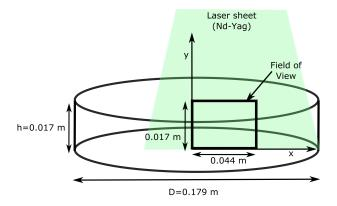
Figure 4: Scheme of the experimental device
