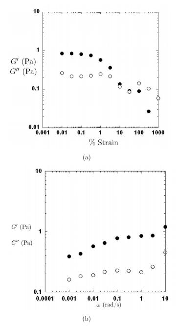
Figure 2: Oscillatory rheometry of the Carbopol gel (a) Variations of G' (Black Circles) and G" (White Circles) as a function of deformation at frequency  $f=\omega/2\pi=0.1$  Hz (b) Pulsation sweep for  $\gamma=1\,\%$ .
