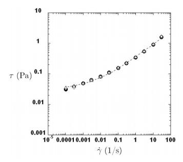
Figure 1: Flow curves of the bulk Carbopol gel for different surfaces (Black circles: sandpaper, White triangles: treated PMMA, White rhombs: treated glass, Dashed line: Herschel-Bulckley model). Rheological properties of the Carbopol gel  $\tau_y = 0.03Pa$  to T = 293K.
