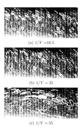
Figure 7: Trajectories (white) obtained by adding recorded images during the time  $t_t$  of the experiment for (a) 1/Y=16.5,  $t_t=360~\rm s$ , (b) 1/Y=25,  $t_t=440~\rm s$  and (c) 1/Y=55,  $t_t=520~\rm s$ .
