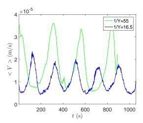
Figure 8: Spatial average over the FOV of the velocity magnitude < V > vs. time for 1/Y = 16.5 and 1/Y = 55
