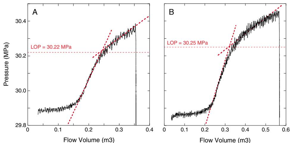
**Figure 7.** Leak-off test (LOT) pressure records for two repeat tests. Leak-off pressure (LOP) is given by the break in slope of the pressure-flow volume curve and is taken to represent the minimum principal stress [e.g., Zoback, 2007].
