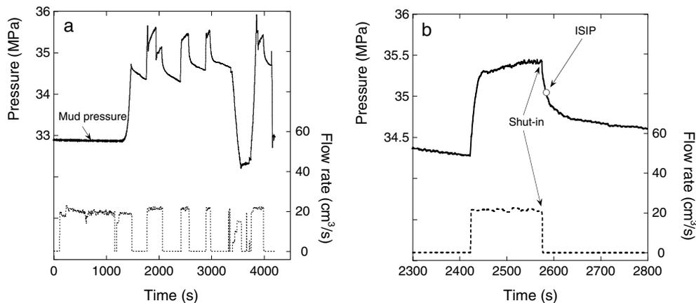
**Figure 6.** Hydraulic fracturing test record for the dual-packer deployment at 876.9 mbsf, showing pressure and fluid pumping rate versus time (positive flow rate indicates injection). (a) Full test record showing three repeat injection cycles. (b) Detailed view of the second injection cycle, showing the instantaneous shut-in pressure (ISIP) taken to indicate the minimum principal stress magnitude.
