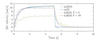
Fig. 11. Bit velocity real data and identified system responses, for initial guess 1.
