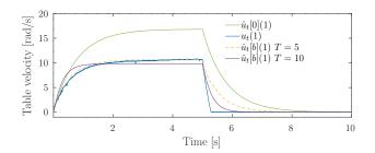
Fig. 17. Real data on the velocity of the table and identified system responses, for initial guess 2.
