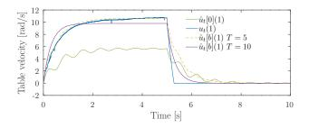
Fig. 10. Real data on the velocity of the table and identified system responses, for initial guess 1.
