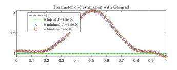
Fig. 3. Estimation of parameter  $a(\cdot)$  using the algorithm (49) for 200 iterations
