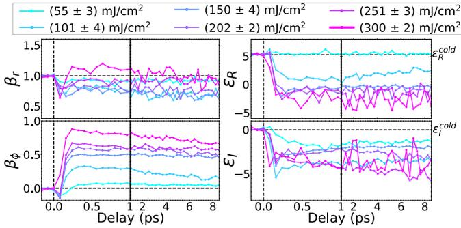
FIG. 10. **Left:** Time evolution of  $\beta_\phi$  and  $\beta_r$  for six different pump intensities. **Right:** Deduced value of the real (top) and imaginary (bottom) parts of the dielectric constant. The value of the initial  $\text{GeS}_2$  was measured by ellipsometry to be  $\epsilon = 5.27 + 0.04 j$
