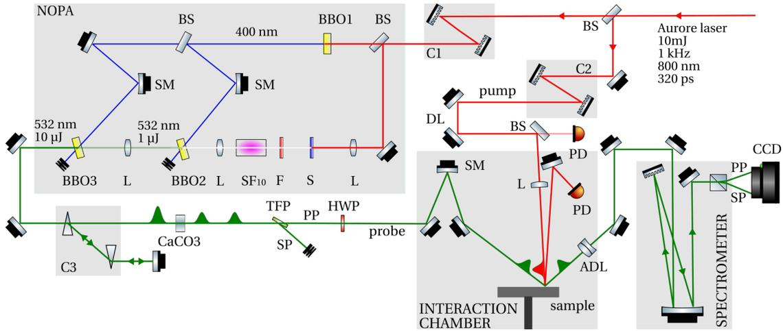
FIG. 9. FDI set-up including the NOPA (BS : beamsplitter, BBO : Beta-Barium Borate crystal, S: sapphire plate, F: 800 nm Notch-filter, SM: spherical mirror, L: Lens, SF<sub>10</sub>: heavy-flint glass, CaCO<sub>3</sub>: calcite crystal, TFP: thin film polarizer, PP: P polarized beam, SP: S polarized beam, C1, C2: double pass grating compressor, C3: prisms compressor, PD: photo-diode, ADL: achromatic doublet lens, DL: delay line, HWP: zero order half wave plate)
