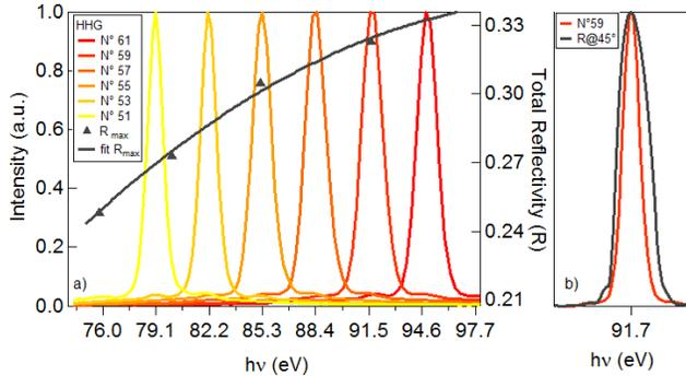
FIG. 12. a) Single harmonic selection with wavelength dependence of the absolute reflectivity of the monochromator. b) Spectral bandwidth of the XUV monochromator at  $45^\circ$  incidence angle and spectral selection of H59.
