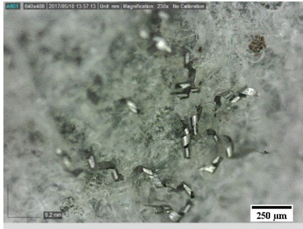
(a) Titanium alloy - f_t = 0.5 \mu\text{m}/\text{tooth} .
