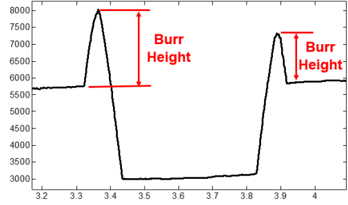
(b) Procedure to measure and compare burr height.
