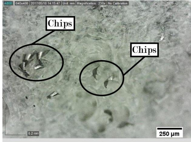
(b) Titanium alloy -  $f_t = 4.0 \mu\text{m}/\text{tooth}$ .
