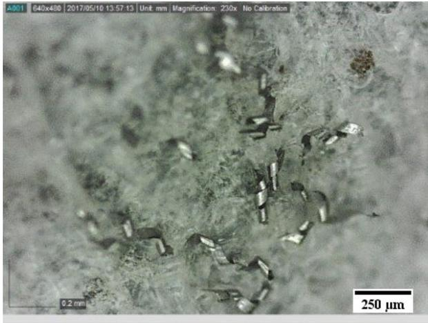
(a) Titanium alloy -  $f_t = 0.5 \mu\text{m}/\text{tooth}$ .
