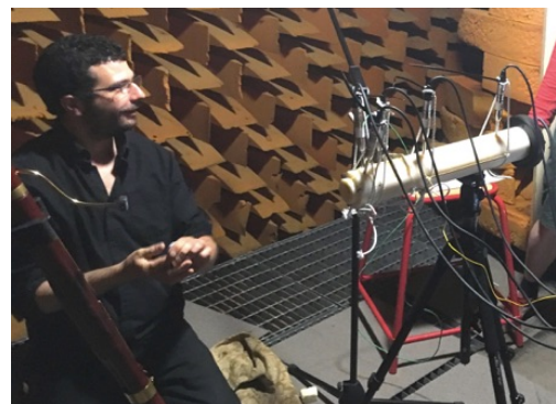
Figure 3. Measurement of a Humeau baroque bassoon with our impedance sensor.
