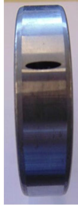
**Fig. 8.** Image of a defect on the ball bearing.**Table 2.** Features of ball bearing and its grease.
