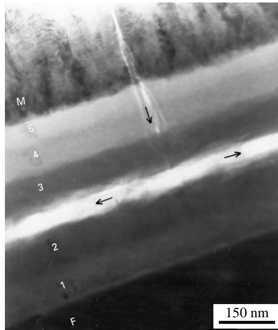
Fig. 6. TEM-image of matrix crack deflection (arrows) in a Nicalon/C(B)/SiC microcomposite [19]
