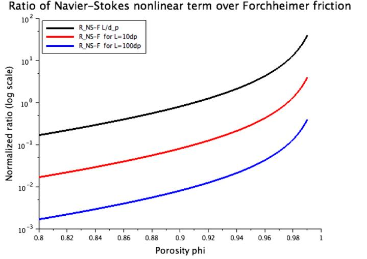
Figure 6: Ratio  $R_{NS/F}$  of the Navier-Stokes nonlinear term over Dupuit-Forchheimer’s inertial friction Eq. (12) in the porosity range  $0.80 \leq \phi < 1$ :  $L = d_p$  (black),  $L = 10 d_p$  (red) and  $L = 100 d_p$  (blue).
