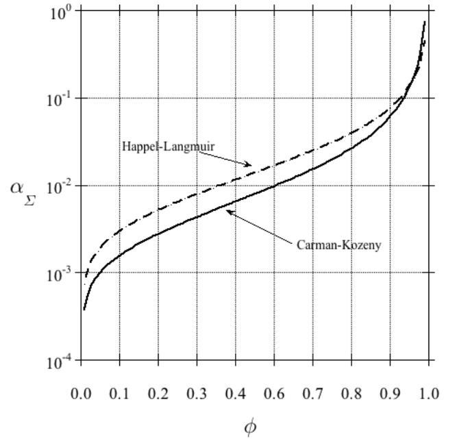
Figure 7: Slip coefficient  $\alpha_\Sigma$  at the interface  $\Sigma$  in (34) for the scaling  $d = 10 d_p$  or  $d = 10 d_f$  and usual  $K_p(\phi_p)$  correlations in  $\Omega_p$  – Solid line: with Kozeny-Carman Eq. (6); Dashed line: with Happel-Langmuir Eq. (7).
