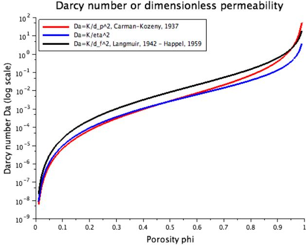
Figure 3: Darcy number (dimensionless permeability)  $Da = K(\phi)/d_p^2$  (red) or  $Da = K(\phi)/\eta^2$  (blue) with Kozeny-Carman's formula Eq. (6) and  $Da = K(\phi)/d_f^2$  (black) with Langmuir-Happel's formula Eq. (7).
