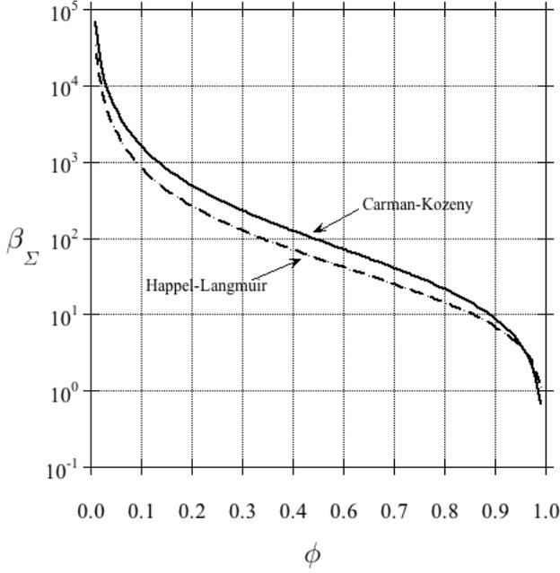
Figure 8: Friction coefficient  $\beta_\Sigma$  at the interface  $\Sigma$  in (34) for the scaling  $d = 10 d_p$  or  $d = 10 d_f$  and usual  $K_p(\phi_p)$  correlations in  $\Omega_p$  – Solid line: with Kozeny-Carman Eq. (6); Dashed line: with Happel-Langmuir Eq. (7).
