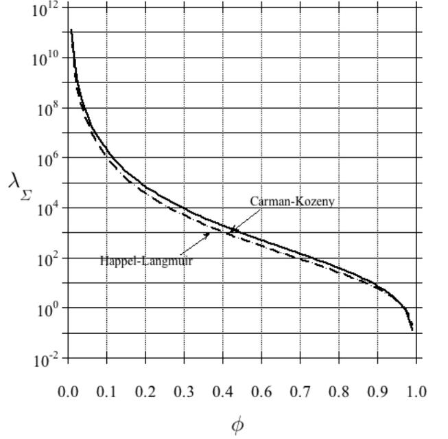
Figure 9: Coefficient of inertial friction  $\lambda_\Sigma \simeq \kappa(\phi_p) \beta_\Sigma$  at the interface  $\Sigma$  in (34) for the scaling  $d = 10 d_p$  or  $d = 10 d_f$ ,  $\kappa(\phi_p)$  correlation (10) from [37, 38] and usual  $K_p(\phi_p)$  correlations in  $\Omega_p$  – Solid line: with Kozeny-Carman Eq. (6); Dashed line: with Happel-Langmuir Eq. (7).
