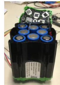
Fig.4. Module of 8 Li-ion LFP cells developed by TYVA ENERGY.
