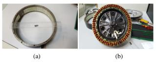
Fig. 5 (a) Outer rotor and magnets of the hub motor; (b) Inner stator of the hub motor.
