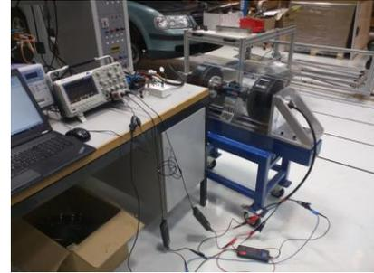
Fig.6 Efficiency test bench with Back-to-Back configuration
