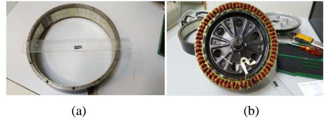
Fig. 5 (a) Outer rotor and magnets of the hub motor; (b) Inner stator of the hub motor.
