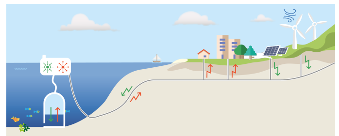
Fig. 1. Station de stockage CAES REMORA
