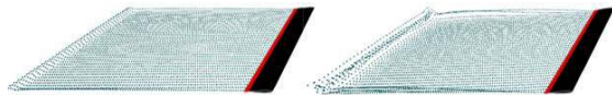
Figure 8. Wake patterns of an instantaneous pitch run from presented VPM for 1° (left) and 5° (right)
