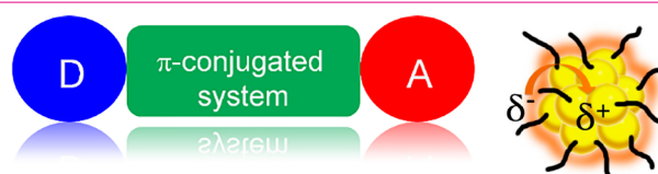
Figure 5. Schematic illustration of (left) a nonlinear optical (NLO), push-pull chromophore and (right) a “ligand-core” NLO-phore with ligand-protected silver and gold clusters.
