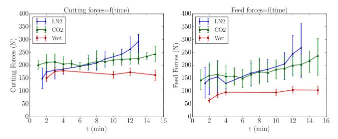
**FIGURE 4.** Comparison between cutting forces components evolution in different cooling conditions: Wet, LN<sub>2</sub> and CO<sub>2</sub>: Cutting forces (left) and Feed forces (right).
