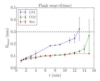
FIGURE 2. Tool flank wear evolution in different cooling conditions: Wet, LN<sub>2</sub> and CO<sub>2</sub>.
