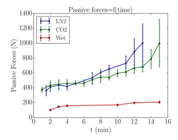
FIGURE 5. Comparison between passive forces evolution in different cooling conditions: Wet, LN<sub>2</sub> and CO<sub>2</sub>.
