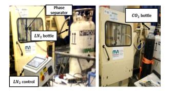
FIGURE 1. Experimental cryogenic systems: LN2 and CO2
