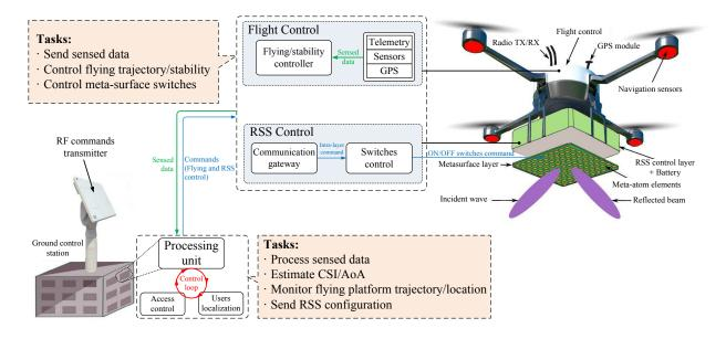
Figure 1. Control architecture of RSS-equipped aerial platforms.
