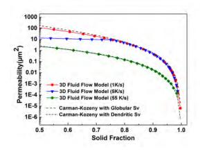
Figure 5: Validation of permeability predicted by present model with the Carman-Kozeny equation for a uniform network of grains with microstructure solidified under the cooling rate of 1K/s, 5K/s and 55K/s.
