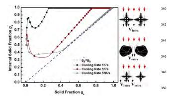
Figure 3: Internal solid fraction evolution within a single grain with<sup>352</sup> a final diameter of 300 µm under three cooling rates along with the schematic diagrams of intra-dendritic, extra-dendritic and both fluid<sub>354</sub> flow types. The dashed line represents the curve  $g'_s = g_s$ .
