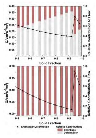
Figure 11: A comparison of Q/V predicted by the 3D dendritic fluid flow model and Eq. 20 as a function of solid fraction for various Fe-C alloys along with the pressure contours at three solid fractions for Fe-0.12wt.% alloy. The required flux to compensate for the peritectic transformation in peritectic grades is also included in the flow predictions of the 3D dendritic fluid flow model. Note that Fig. 10(b1) and (b2) share the same color bar.
