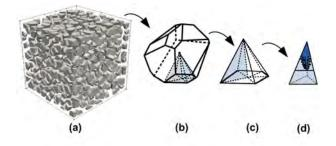
Figure 1: (a) Meso-scale simulation domain containing 1000 grains; (b) Single Voronoi grain; (c) Polyhedral structure; (d) Tetrahedron with an illustrative schematic of the equiaxed-dendritic microstructure.
