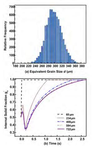
Figure 6: (a) Equivalent grain size d distribution within the semisolid domain and (b) the variation in  $g_s'$  for five grains containing different sizes.
