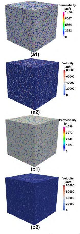
Figure 10: Variations in permeability (-1) and local velocity (-2) 11 within a semisolid domain at (a) $g_s=0.70$  and (b)  $g_s=0.84$ . The grain size was 500 µm, and the cooling rate was 5 K/s
