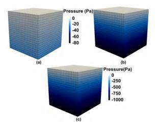
Figure 4: Pressure distribution within a domain containing 8000 grains at  $g_s$ =0.60 solidified under three cooling rates: (a) CR=1K/s, (b) CR=5K/s and (c) CR=55K/s. Note that Fig. 4(a) and (b) share the same color bar.
