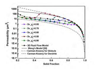
Figure 9: Influence of  $S_v$  calculated based on different internal solid fractions on the prediction of the permeability within mushy zonesis via Carman-Kozeny equation . The permeability calculated via the Carman-Kozeny for Globular and Dendritic cases, as well as via Wang's model [20] is provided for comparison purposes. Wang's <sup>620</sup> model was applied using a grain size of 300 µm and a dendrite envelope sphericity  $\phi_e = 1$ .
