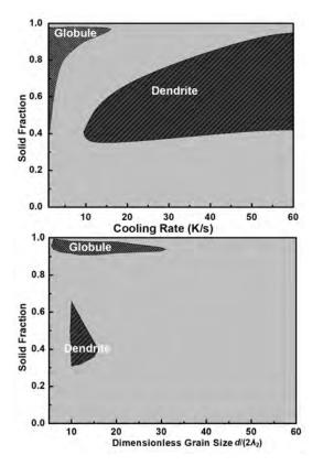
Figure 8: Permeability map as a function of solid fractions and (a) cooling rate as well as (b) dimensionless grain size,  $d/(2 \cdot \lambda_2)$ .
