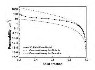
Figure 7: Variations of permeability as a function of solid fraction for a semisolid domain containing both intra-dendritic and extradendritic flow.
