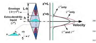
Figure 2: Schematic diagram of two facing tetrahedrons, the velocity profile of fluid passing through the inter- and extra- dendritic regions, and the corresponding 3-node 2D triangular element. The velocity profiles for the cases with only intra-dendritic and only extradendritic flow are also shown.
