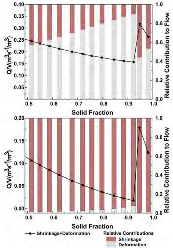
Figure 12: A comparison of the  $Q/V$  predicted by the 3D dendritic fluid flow model taking into account both solidification shrinkage and deformation. Strain rates of  $0.1 \text{ s}^{-1}$  (upper) and  $0.001 \text{ s}^{-1}$  (lower) are examined.
