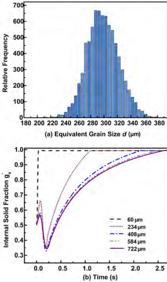
Figure 6: (a) Equivalent grain size  $d$  distribution within the semisolid domain and (b) the variation in  $g_s$  for five grains containing different sizes.
