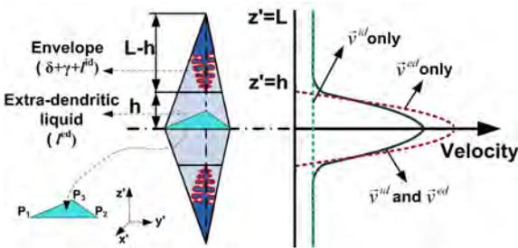
Figure 2: Schematic diagram of two facing tetrahedrons, the velocity profile of fluid passing through the inter- and extra- dendritic regions, and the corresponding 3-node 2D triangular element. The velocity profiles for the cases with only intra-dendritic and only extra-dendritic flow are also shown.
