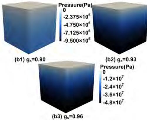
Figure 11: A comparison of  $Q/V$  predicted by the 3D dendritic fluid flow model and Eq. 20 as a function of solid fraction for various Fe-C alloys along with the pressure contours at three solid fractions for Fe-0.12wt.% alloy. The required flux to compensate for the peritectic transformation in peritectic grades is also included in the flow predictions of the 3D dendritic fluid flow model. Note that Fig. 10(b1) and (b2) share the same color bar.
