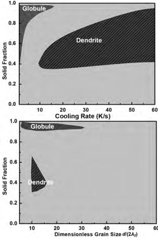
Figure 8: Permeability map as a function of solid fractions and (a) cooling rate as well as (b) dimensionless grain size,  $d/(2 \cdot \lambda_2)$ .
