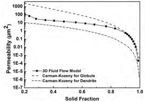
Figure 7: Variations of permeability as a function of solid fraction for a semisolid domain containing both intra-dendritic and extra-dendritic flow.
