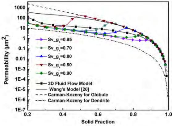
Figure 9: Influence of  $S_v$  calculated based on different internal solid fractions on the prediction of the permeability within mushy zone via Carman-Kozeny equation. The permeability calculated via the Carman-Kozeny for Globular and Dendritic cases, as well as via Wang's model [20] is provided for comparison purposes. Wang's model was applied using a grain size of 300  $\mu\text{m}$  and a dendrite envelope sphericity  $\phi_e = 1$ .
