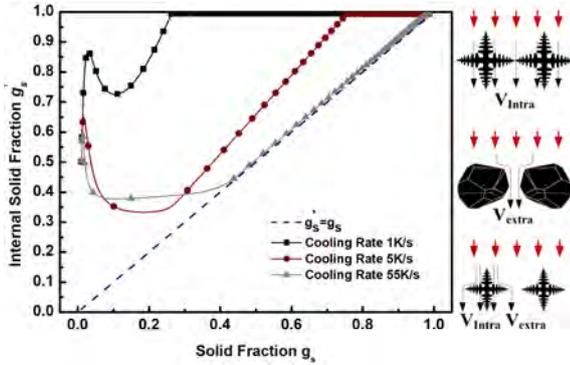
Figure 3: Internal solid fraction evolution within a single grain with a final diameter of 300  $\mu\text{m}$  under three cooling rates along with the schematic diagrams of intra-dendritic, extra-dendritic and both fluid flow types. The dashed line represents the curve  $g'_s = g_s$ .
