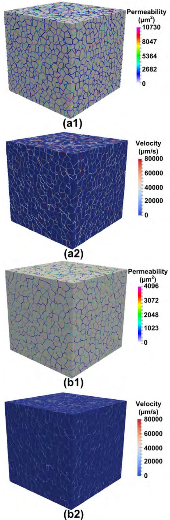
Figure 10: Variations in permeability (-1) and local velocity (-2) within a semisolid domain at (a)  $g_s=0.70$  and (b)  $g_s=0.84$ . The grain size was 500  $\mu\text{m}$ , and the cooling rate was 5 K/s
