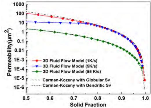
Figure 5: Validation of permeability predicted by present model with the Carman-Kozeny equation for a uniform network of grains with microstructure solidified under the cooling rate of 1K/s, 5K/s and 55K/s.
