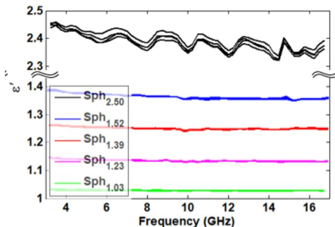
Fig. 4. Real part of the relative permittivity of the meshed spheres presented in Table I as a function of the frequency. For the sake of comparison, the results obtained with a higher index sphere S<sub>2.5</sub><sup>1.15</sup> (presented in Table II) are also shown. For each sphere, 4 permittivity determinations are made, corresponding to 4 orientations of the sphere.
