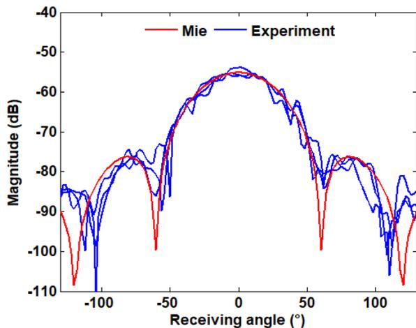
Fig 9. Magnitudes of the measured fields scattered by the 35 mm diameter meshed sphere  $S_{1.03}$  with comparison to the Mie simulation of an equivalent homogeneous sphere of permittivity  $1.03+j0.002$  at 12 GHz.
