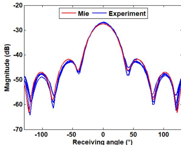
Fig. 8. Magnitudes of the measured fields scattered by the 35 mm diameter meshed sphere  $S_{2.5}^{1.15}$  with comparison to the Mie simulation of an equivalent homogeneous sphere of permittivity  $2.35 + j0.09$  at 12 GHz
