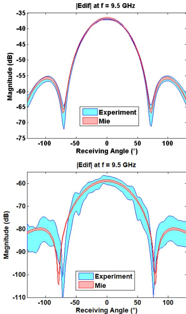
Fig. 10. Representation of the uncertainty estimations for the  $S_{1.39}$  sphere (top) and the  $S_{1.03}$  sphere (bottom). The cyan zone represents the experimental scattered field with the standard deviation observed from 500 repetitive measurements. The light red zone represents the variations corresponding to a Monte-Carlo computation: 500 permittivity values taken from the extreme range values of permittivities are used as inputs to the Mie simulation.
