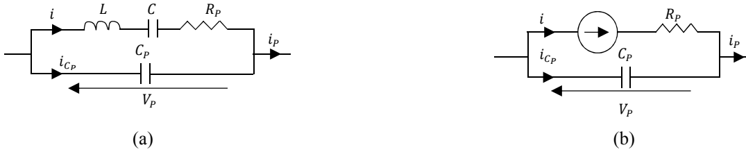
Fig. 2: Electrical model for PRs, (a) Circuit model [15], (b) Electrical model in inductive region.
