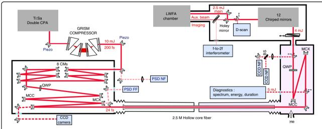
Fig. 1 Schematics of the vacuum-integrated stretched flexible hollow fiber pulse compressor setup. PSD photosensitive detector, NF near field, FF far field, piezo piezo-driven mirror mounts, MCX convex mirror, MCC concave mirror, QWP quarter-wave plate
