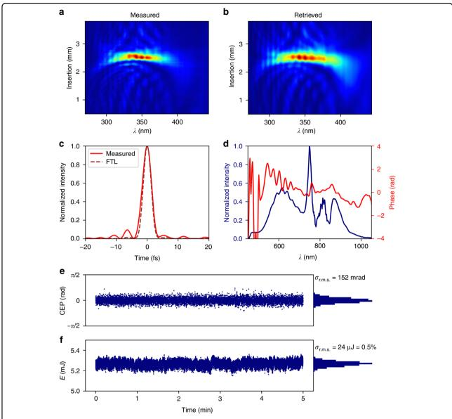
Fig. 2 D-scan measurement for 1.3 bar helium pressure. Measured (a) and retrieved (b) d-scan traces. Reconstructed temporal profile (c): the retrieved temporal pulse profile is shown in red (3.4 fs FWHM). The ideal Fourier transform-limited shape (2.9 fs FWHM) is indicated by the brown dotted line. Measured spectral intensity and phase (d). Relative CEP stability (each point averaged over 30 shots) (e) and pulse energy at the fiber exit (f), both measured over 5 min
