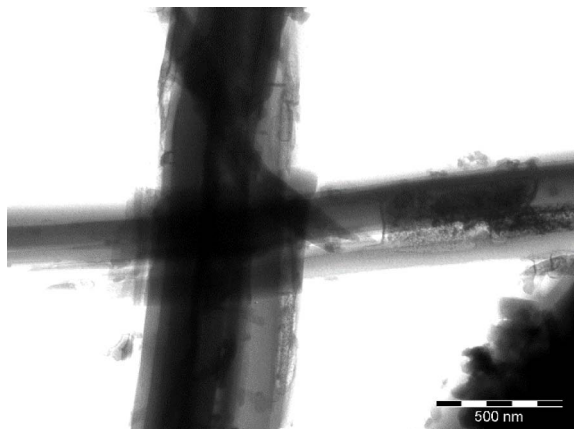
Figure 3. Electron micrograph for \text{Per}_2[\text{Au}(\text{mnt})_2] in the absence of growth controlling agent (bar = 500 nm).
