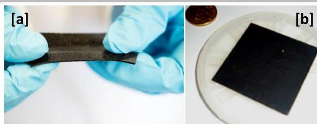
**Figure 10.** [a] Composite containing 5% wt. of TTF-TCNQ nanoparticles in a space-qualified resin, thickness: 0.4 mm. ©Frédéric MALIGNE/LCC/CNRS Photothèque, Copyright (2018), with permission from CNRS Photothèque. [b] Alumina substrate (5 cm  $\times$  5 cm) covered by a continuous deposit of TTF-TCNQ nanoparticles, thickness =  $90.00 \pm 0.04 \mu\text{m}$ . Reproduced from ref.<sup>[14f]</sup>, Copyright (2013), with permission from the American Chemical Society.
