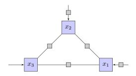
Suppose the system operator wishes to reconstruct the voltage phase angles at  $x_1, x_2, x_3$  and that noisy active power flow measurements are available at the grey squares. This can be formulated as  $y, w \in \mathbb{R}^5, x \in \mathbb{R}^3$  with noisy measurements, so that y = Hx + Fa + w with
