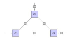
Suppose the system operator wishes to reconstruct the voltage phase angles at  $x_1, x_2, x_3$  and that noisy active power flow measurements are available at the grey squares. This can be formulated as  $y, w \in \mathbb{R}^5, x \in \mathbb{R}^3$  with noisy measurements, so that y = Hx + Fa + w with
