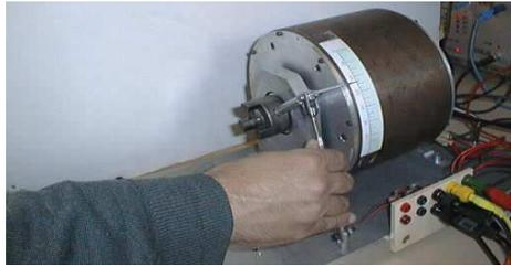
Fig 6:  $L_d$ ,  $L_q$  and  $M$  measurement [32]
