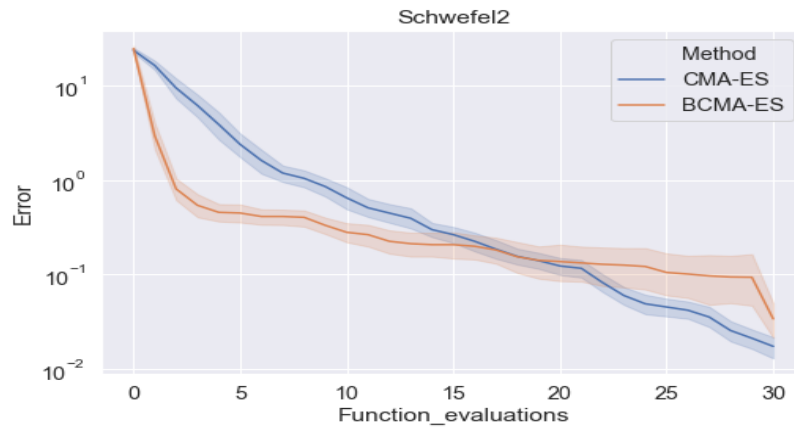
Fig. 19. Convergence for the schwefel2 function with a starting point at [-5,-5]
