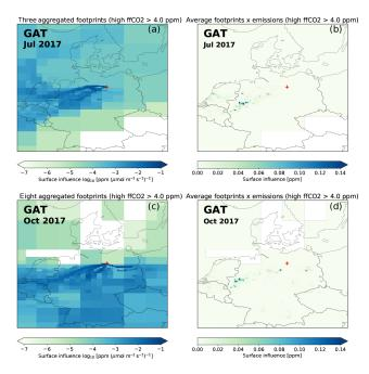
**Figure 9.** Aggregated footprints with elevated ffCO<sub>2</sub>, and the corresponding surface influences for Gartow in July 2017 (**a–b**) and October 2017 (**c–d**), based on the EDGAR version 4.3.2 emission inventory. Note the logarithmic colour scale in the aggregated footprint maps.
