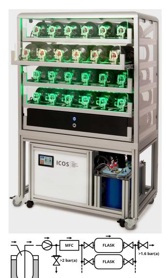
**Figure 2.** Photograph of the ICOS flask sampler with a schematic flow diagram.
