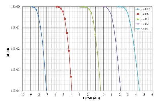
Figure 7: Performance evaluation of the enhanced turbo code in AWGN channel in terms of BLock Error Rate vs Es/N0. **QPSK modulation**, information block size K = 600 bits, 8 decoding iterations of the Max-log-MAP algorithm, tail-biting termination.
