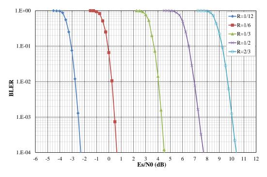
Figure 13: Performance evaluation of the enhanced turbo code in AWGN channel in terms of BLock Error Rate vs Es/N0. **16QAM modulation**, information block size K = 600 bits, 8 decoding iterations of the Max-log-MAP algorithm, tail-biting termination.
