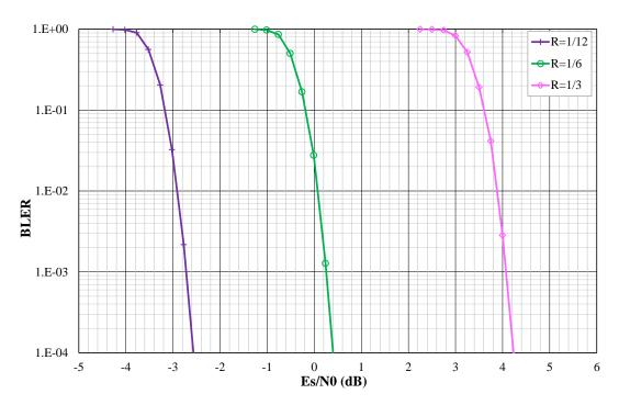
Figure 14: Performance evaluation of the enhanced turbo code in AWGN channel in terms of BLock Error Rate vs Es/N0. **16QAM modulation**, information block size K = 992 bits, 8 decoding iterations of the Max-log-MAP algorithm, tail-biting termination.
