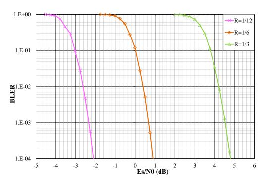
Figure 12: Performance evaluation of the enhanced turbo code in AWGN channel in terms of BLock Error Rate vs Es/N0. **16QAM modulation**, information block size K = 400 bits, 8 decoding iterations of the Max-log-MAP algorithm, tail-biting termination.
