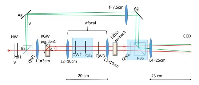
Fig. 1 Experimental set-up allowing the OAM study in the far field. The CD-field in position 1 is transported without modification in position 2 by the L2-L3 afocal telescope.
