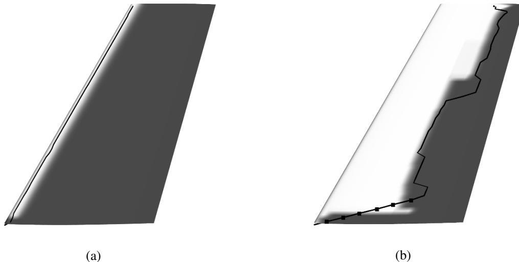
Fig. 1 Intermittency contours (light and dark corresponds respectively to \gamma = 0 and \gamma = 1 ) at the suction (a) and pressure (b) sides. The black line depicts the transition location predicted by 3C3D by means of AHD/C1 transition criteria. Black squares depict transition by turbulent wedge in 3C3D. Flow is coming from left to right.
