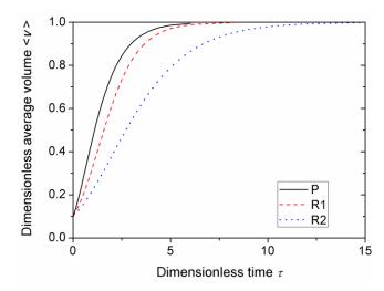
**Fig. 2.** Dimensionless average aggregate volume  $\langle v \rangle$  as function of dimensionless time  $\tau$  for three different functions g(v) and initial log-normal size distribution with  $\langle v \rangle_0 = 0.1$  and  $\sigma = 1.5$ . The case R2 is calculated for a=b=1.
