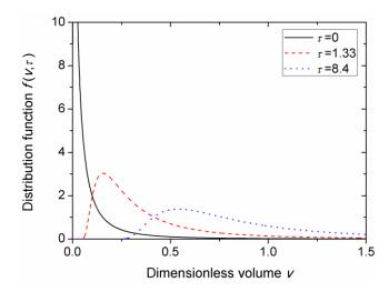
Fig. 4. Aggregate size distribution for the R1-case with  $\langle v \rangle_0 = 0.1$ ,  $\sigma = 1.5$  and at the dimensionless times  $\tau$ , covering the whole range of the average volume  $\langle v \rangle_0 \leq \langle v \rangle \lesssim 1$ .
