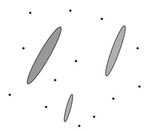
**Fig.1.** Sketch of the aggregates, which can either be stationary or perform an angular motion depending on the applied magnetic field. Dots around the aggregates stand for individual magnetic particles.
