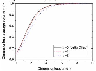
Fig. 3. Dimensionless average aggregate volume  $\langle v \rangle$  as function of dimensionless time  $\tau$  for the R1-case and initial log-normal size distribution with  $\langle v \rangle_0 = 0.1$  and three different values  $\sigma$  of the distribution width.
