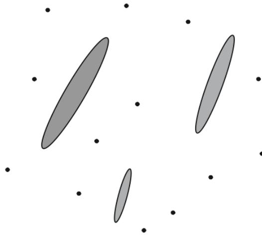
**Fig.1.** Sketch of the aggregates, which can either be stationary or perform an angular motion depending on the applied magnetic field. Dots around the aggregates stand for individual magnetic particles.
