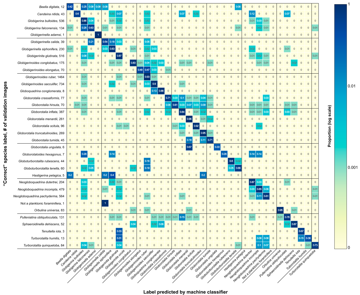
Figure 4. The machine confusion matrix, showing results from the validation set, which contains 80% of the images with high-quality labels from the combined YPM coretop data set and the Buckley data set. The y axis shows the “correct” species labels followed by the number of representative images in the validation set. The x axis shows the corresponding predicted labels, with each matrix cell showing the proportion of validation objects identified as each species (e.g., 86% of the 536 validation images of G. bulloides were correctly identified as G. bulloides and 4% were incorrectly identified as G. falconensis ). The color map is on a log-scale and shows higher (bluer/darker) vs. lower proportions (yellow/lighter).
