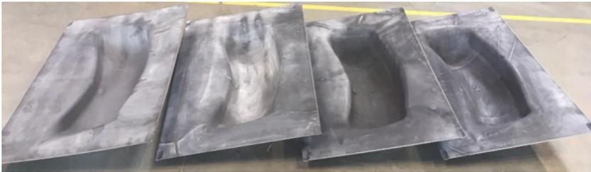
**Figure 14: Four consecutive IR formed sheets after the trimming of the cold frame area**
