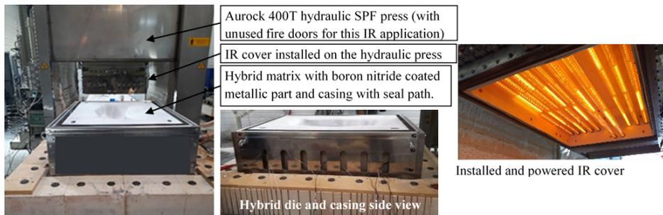
**Figure 10: Tool installation on the 400T Aurock dual (Conventional/IR HF/SPF) hydraulic press.**
