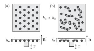
FIG. 1. (a) Top and (b) side views of a confined system of magnetic granular material. At fixed number of particles and magnetic field  $\bf B$ , decreasing the degree of confinement, i.e., the cell height, leads to the formation of labyrinthine patterns.  $\Gamma$  denotes the dimensionless acceleration of the vibrations.
