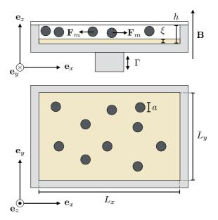
FIG. 2. Side and top view of the experimental setup that is reproduced numerically. An  $L_x \times L_y \times h$  cell, enclosing N spherical beads of diameter a, is vertically vibrated with a dimensionless acceleration  $\Gamma$ . The system is placed in a vertical magnetic field  $\mathbf{B}$  which induces magnetic dipolar forces  $\mathbf{F}_m$  between the particles.
