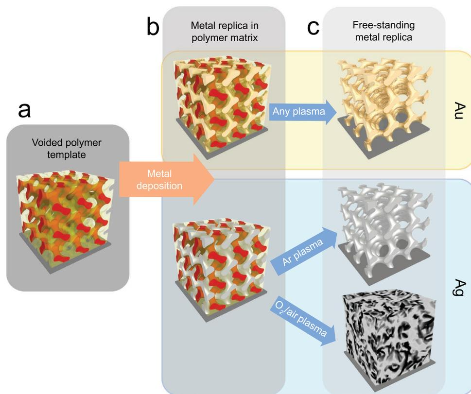
**Figure 1.** Schematic diagram of the sample fabrication.<sup>[25]</sup> a) Starting from a voided ISO triblock terpolymer template, b) Au (top) or Ag (bottom) are electrodeposited into the voided network. c) The polymer template is then removed by plasma etching, resulting in a free-standing, metallic gyroid replica. For Ag, only Ar plasma etching results in a stable nanostructure, while for gold any plasma (Ar, O<sub>2</sub>, or air) can be employed.
