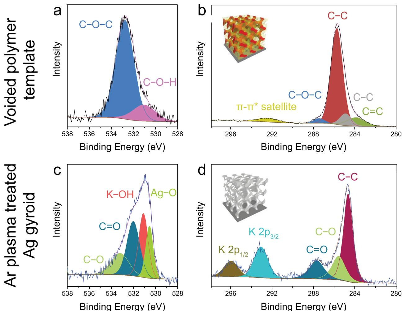
**Figure 4.** XPS analysis of carbon and oxygen contamination on Ag gyroid surfaces. High-resolution XPS spectra of the O 1s and C 1s regions of a,b) a voided ISO gyroid terpolymer film and c,d) an Ar plasma-cleaned Ag gyroid. The colored shading corresponds to fits assuming binding energies of the indicated bonds.
