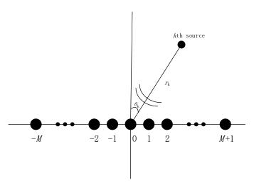
Fig. 1. Near-field source localization with ULA.
