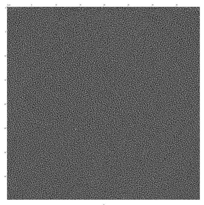
FIG. S4. Large-scale atomic force microscope image,  $40 \times 40 \ \mu m^2$  with a  $2048 \times 2048$  points, of 25 nm Ge deposited on UT-SOI and annealed at  $480^{\circ}$ C for 45 minutes. This image was used for Minkowski analysis of experimental patterns and for the hyperuniformity analysis.
