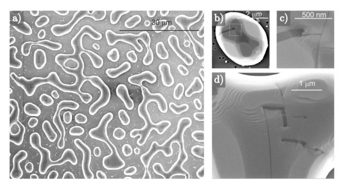
FIG. S3. a) Scanning electron micrograph of 500 nm Ge on UT-SOI after 6 hours annealing at 800°C. b) Detail of a dewetted island with large facets. c) Zoom of the area highlighted by a white square in b). d) Detail of facets, terraces and step bunching.
