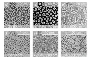
FIG. S2. Size and morphology tuning. SEM images of  $Si_{1-x}Ge_x$  layers of thickness h deposited on UT-SOI and annealed for a time t at temperature T: a) x=1, h=50 nm, t=45 min,  $T=750^{\circ}C$ ; b) x=0.3, h=100 nm, t=150 min,  $T=800^{\circ}C$ ; c) x=1, h=1000 nm, t=4 h,  $T=800^{\circ}C$ ; d) x=1, h=10 nm, t=30 min,  $T=450^{\circ}C$ ; e) x=0.3, h=200 nm, t=1 h,  $T=800^{\circ}C$ . f) x=1, h=1500 nm, t=4 h,  $T=800^{\circ}C$ .
