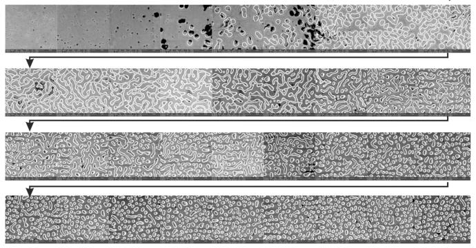
FIG. S1. Scanning electron micrographs (SEM) displaying the morphological evolution (from the edge of the sample, left panel, towards its center, right panel) of 150 nm  $Si_{0.7}Ge_{0.3}$  on UT-SOI after 4 hours annealing at 800°C. Another example from a different sample is provided as a separate high-resolution Supplementary File 1 where optical microscopy shows that the change in morphology occurs over about 0.5 mm from the edge.
