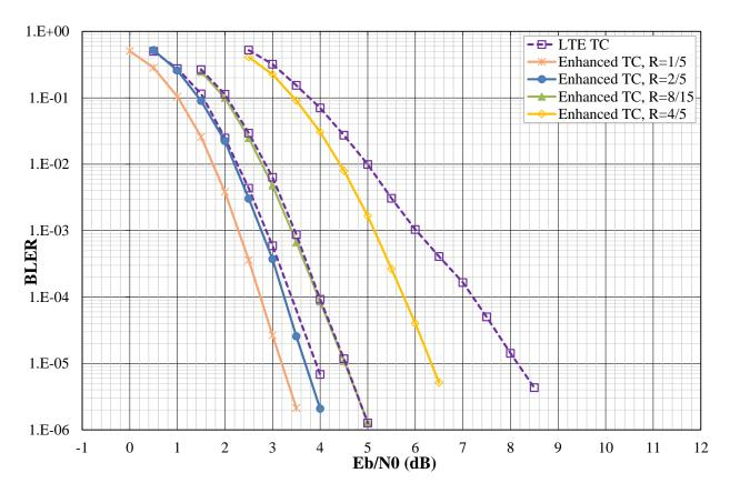
Figure 6: Performance comparison of the improved turbo code with the LTE turbo code in AWGN channel for coding rates 1/5, 2/5, 8/15, and 4/5 in terms of BLock Error Rate vs Eb/N0.
