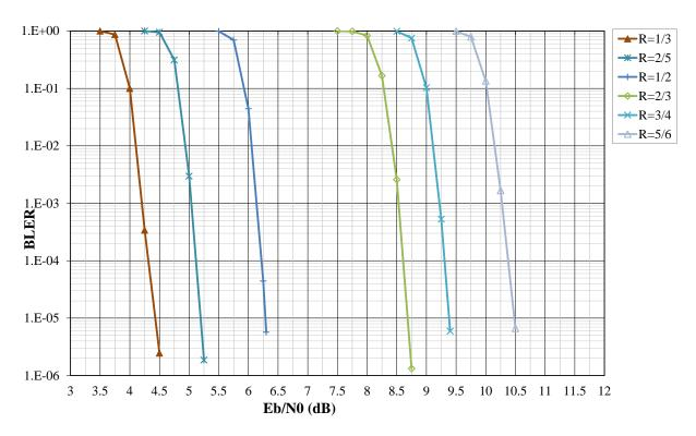
Figure 5: Performance evaluation of the improved turbo code in AWGN channel in terms of BLock Error Rate vs Eb/N0.
