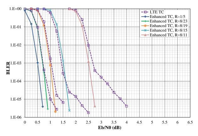
Figure 11: Performance comparison of the improved turbo code with the LTE turbo code in AWGN channel for coding rates 1/5, 8/23, 8/19, 8/15, and 8/11 in terms of BLock Error Rate vs Eb/N0.
