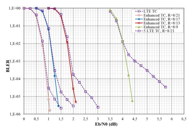
Figure 14: Performance comparison of the improved turbo code with the LTE turbo code in AWGN channel for coding rates 8/21, 8/17, 8/13, and 8/9 in terms of BLock Error Rate vs Eb/N0.
