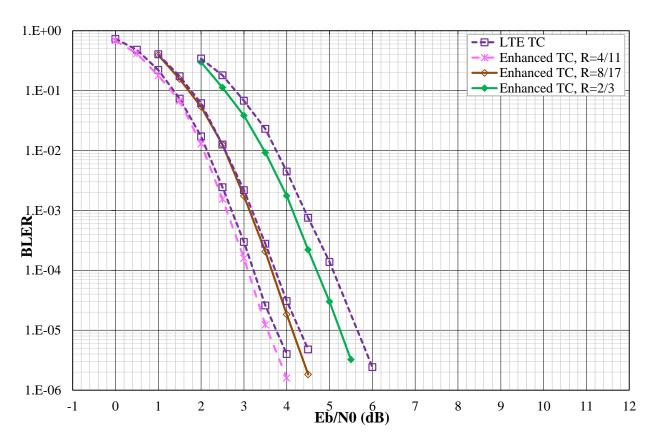
Figure 9: Performance comparison of the improved turbo code with the LTE turbo code in AWGN channel for coding rates 4/11, 8/17, and 2/3 in terms of BLock Error Rate vs Eb/N0. QPSK modulation, block size K=96 bits, 8 decoding iterations of the Max-Log-MAP algorithm, tail-biting termination.
