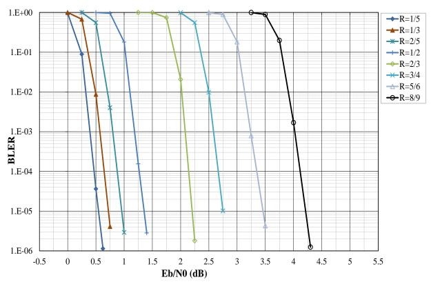
Figure 4: Performance evaluation of the improved turbo code in AWGN channel in terms of BLock Error Rate vs Eb/NO.
