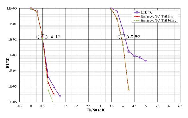
Figure 3: Performance comparison of the improved turbo code (when using tail bits or tail-biting termination) with the LTE turbo code in AWGN channel for coding rates 1/3 and 8/9 in terms of BLock Error Rate vs Eb/NO.
