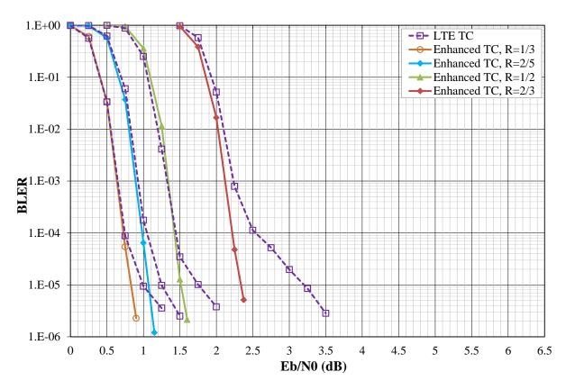
Figure 12: Performance comparison of the improved turbo code with the LTE turbo code in AWGN channel for coding rates 1/3, 2/5, 1/2, and 2/3 in terms of BLock Error Rate vs Eb/N0.
