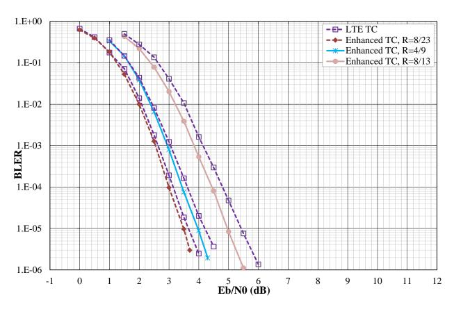
Figure 8: Performance comparison of the improved turbo code with the LTE turbo code in AWGN channel for coding rates 8/23, 4/9, and 8/13 in terms of BLock Error Rate vs Eb/N0. QPSK modulation, block size K=96 bits, 8 decoding iterations of the Max-Log-MAP algorithm, tail-biting termination.
