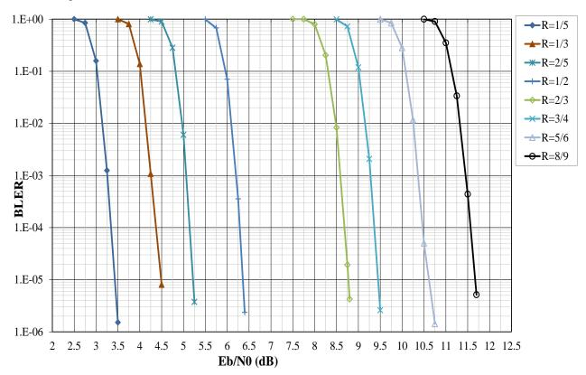
Figure 2: Performance evaluation of the improved turbo code in AWGN channel in terms of BLock Error Rate vs Eb/N0.
