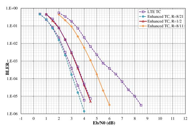
Figure 10: Performance comparison of the improved turbo code with the LTE turbo code in AWGN channel for coding rates 8/21, 1/2, and 8/11 in terms of BLock Error Rate vs Eb/N0. QPSK modulation, block size K=96 bits, 8 decoding iterations of the Max-Log-MAP algorithm, tail-biting termination.
