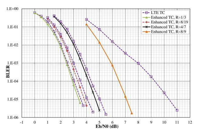
Figure 7: Performance comparison of the improved turbo code with the LTE turbo code in AWGN channel for coding rates 1/3, 8/19, 4/7, and 8/9 in terms of BLock Error Rate vs Eb/N0.
