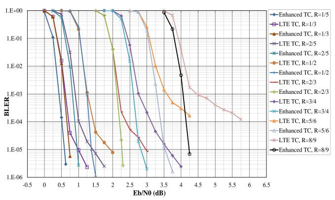
Figure 1: Performance comparison of the improved turbo code with the LTE turbo code in AWGN channel in terms of BLock Error Rate vs Eb/N0. QPSK modulation, block size K = 6000 bits (K = 6016 bits for LTE TC), 8 decoding iterations of the Max-Log-MAP algorithm, tail-biting termination.
